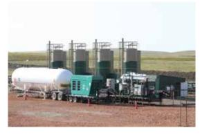
VOCs by liquefying and storing them. These valuable NGLs and purified wellhead natural gas streams are diverted away from flare stacks, resulting in significantly improved environmental performance and the opportunity to reduce production costs and increase revenue. GTUIT CORE™ systems in successful operation in the Bakken oil fields today.
