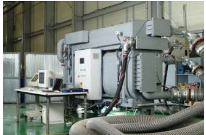
Test of Absorption Chiller
